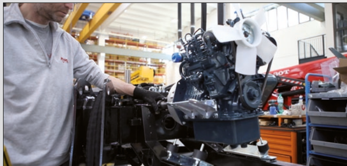
Endothermic diesel engine replacing the petrol engine (models up to 20m only).
