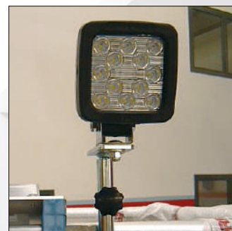
Work light in the basket.
