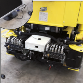
Location and remote diagnostic device applied to the platform. Allows remote diagnosis.
