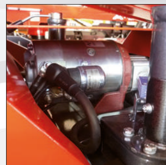
Emergency electric pump, allows to bring to the operator in basket to the ground in case of endothermic motor failure.
