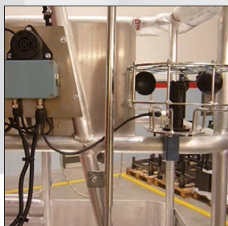
Wind speed control device, with alarm.
