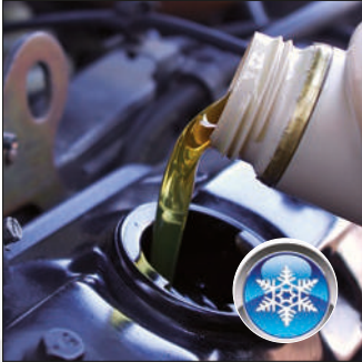
ARTICO synthetic oil load for very cold climates (suggested for temperatures starting from -5° C).
