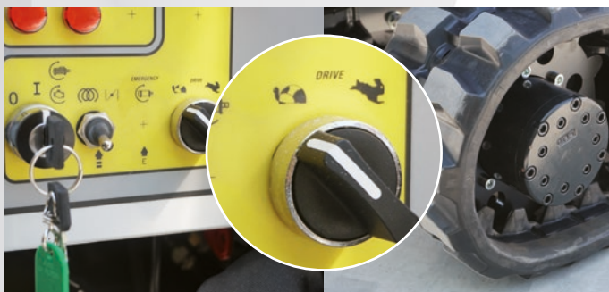
Track transmission with slow/fast double speed (only models up to 18m in height).
