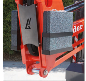
Application of plate-holder frame with 4 plates provided to reduce the pressure on the ground.
